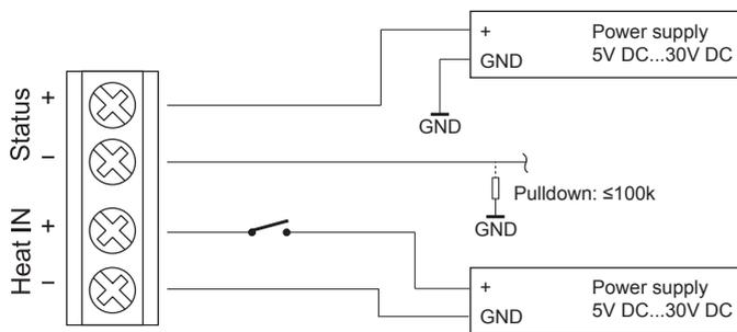
Fig. 3 ARC trigger and status connection
