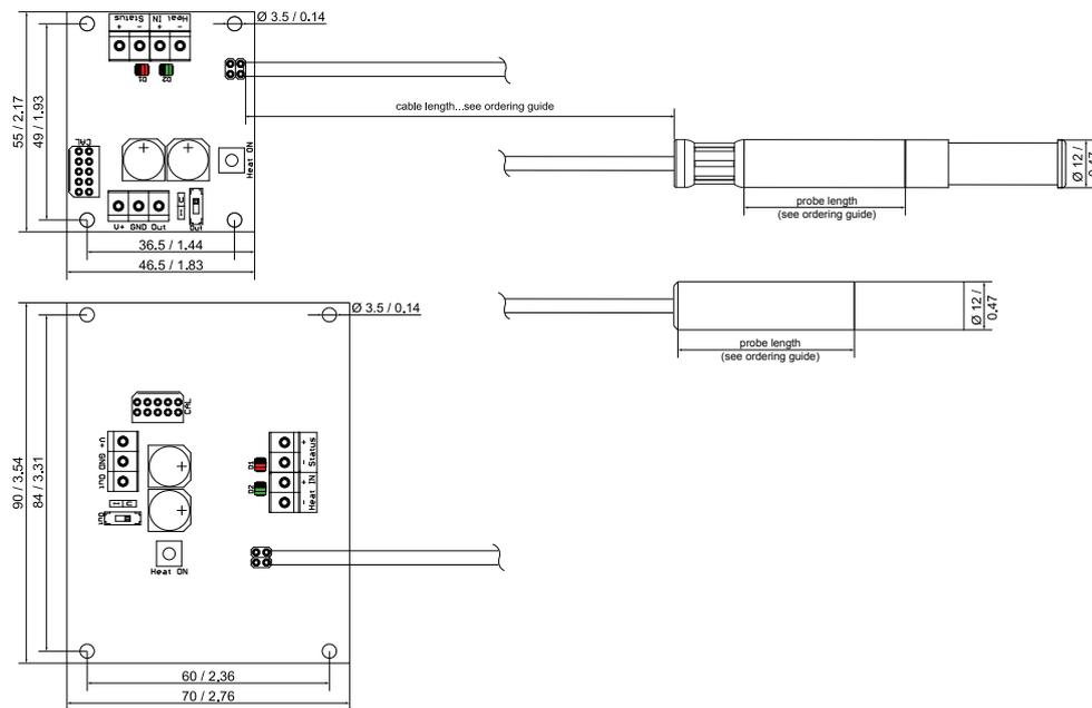
Fig. 1 Dimensions of EE1900
